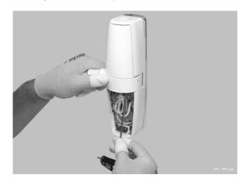
access to adjustment screw when locking screw removed
